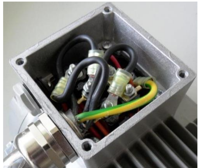
Fig. 30: Wiring on the motor connection box
