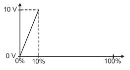
The setting of the parameter *Offset* **585** to 0.00% and the parameter *Amplification* **586** to 1000.0% means that the output signal:
