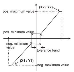
With tolerance band and minimum value
