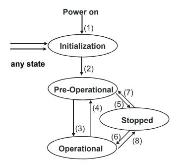
After Power On and initialization, the slaves are in the Pre-Operational state. The transition (2) is automatic. The system bus master (frequency inverter or PLC/PC) triggers the transition (3) to Operational state.
