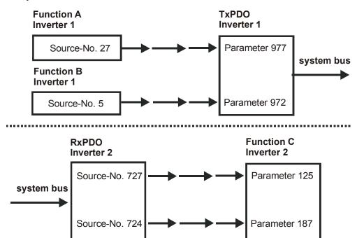
Example 2 displays the same situation as Example 1. But now, the functions A and B are in frequency inverter 1 and function C in frequency inverter 2. The connection is done via a TxPDO in frequency inverter 1 and a RxPDO in frequency inverter 2. Thus, the parameterization for this connection is:
