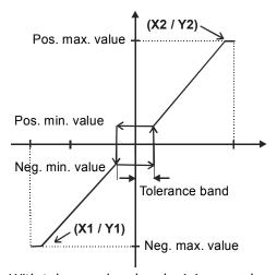
With tolerance band and minimum value
