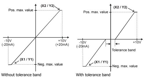
The *Minimum Frequency* **418** or the *Minimum reference percentage* **518** set in the factory extend the parameterized tolerance band to the hysteresis.
