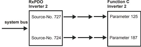
Example 2 displays the same situation as Example 1. But now, the functions A and B are in frequency inverter 1 and function C in frequency inverter 2. The connection is done via a TxPDO in frequency inverter 1 and a RxPDO in frequency inverter 2. Thus, the parameterization for this connection is:
