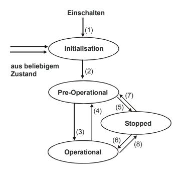
After Power On and the initialization, the slaves are in the Pre-Operational state. The transition (2) is automatic. The system bus master (frequency inverter or PLC/PC) triggers the transition (3) to Operational state.
