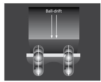
Fig. 6 Ball Drifting
